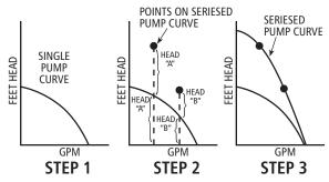
Seriesed Pump Curve Construction Figure 30
