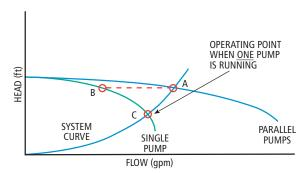
Single Pump Operation – Paralleled Installation Figure 9
