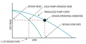
Two Parallel Pump System Operation Figure 4
