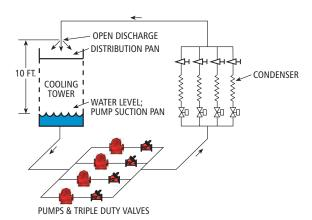
Typical Large Condenser Water System Figure 17
