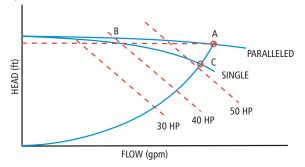
BHP Increase During Single Pump Operation Figure 10
