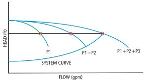
Three Parallel Pumps; Open System Figure 18
