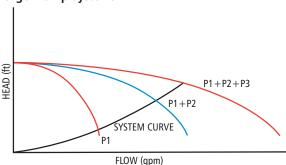
Three Pump Paralleled Pump Curve Construction Figure 13
