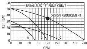
Paralleled "B" Pump Curve Figure 22
