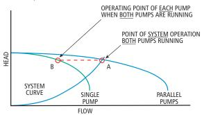
Paralleled Pump System Operation Figure 8
