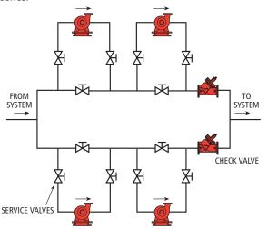
Basic Paralleled & Seriesed Pump Installation Figure 38
