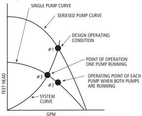
Single Pump Operation – Seriesed Installation Figure 32
